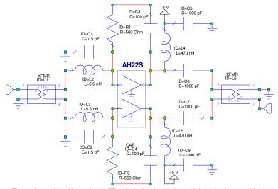
The transformers, L1 and L6, used on the WJ evaluation board are handwound baluns using these materials: 6 turns bifilar wire (MWS B2383211) around a ferrite core (TDK, H5C2-T3.1-1.3-1.3). An SMT transformer (M/A Com ETC1-1-13) can also be used.
